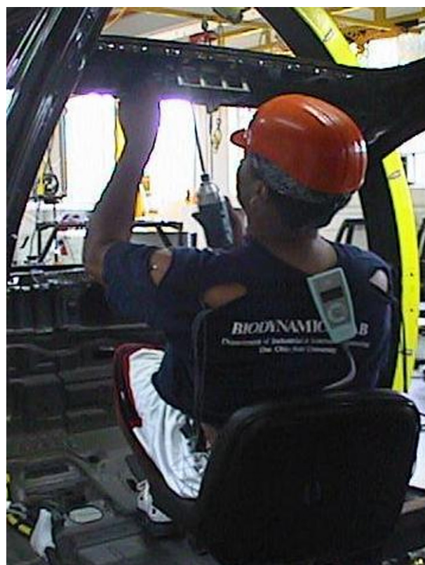
Fig. 3. Cantilever chair in use for assembly task.
