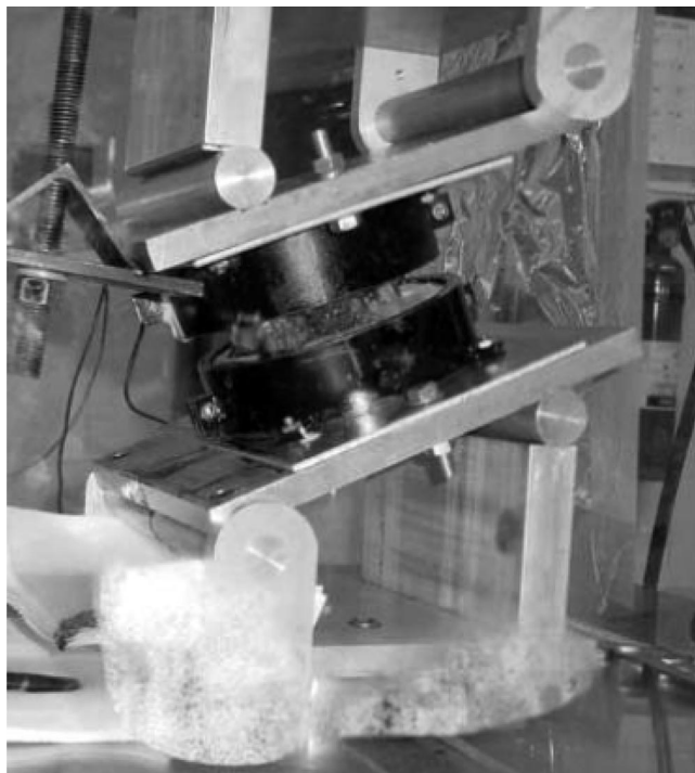
Figure 2. Illustration of loading jig with specimen attached, inside environmental chamber.
