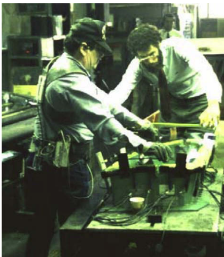
Fig. 1. The traditional approach to measuring load moment entailed multiplying a measurement of the horizontal distance between the base of the spine and the object's center of mass by the weight of the object.
