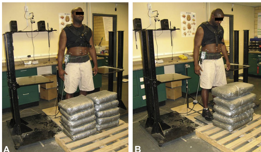
Fig. 1. Test set-up for 10 bags weighing 21.4 kg (A), and 5 bags weighing 42.7 kg bags (B).
