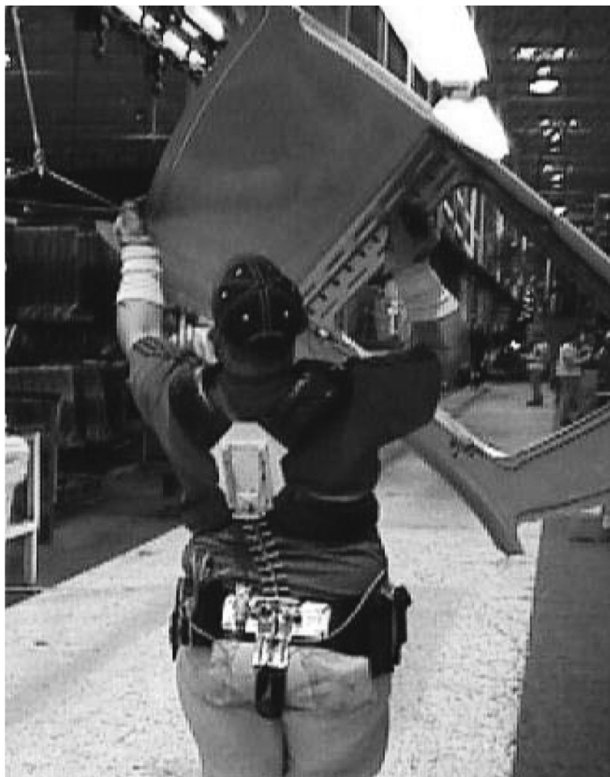
Figure 1. The lumbar motion monitor (LMM) worn by a worker performing a manual material handling job.
