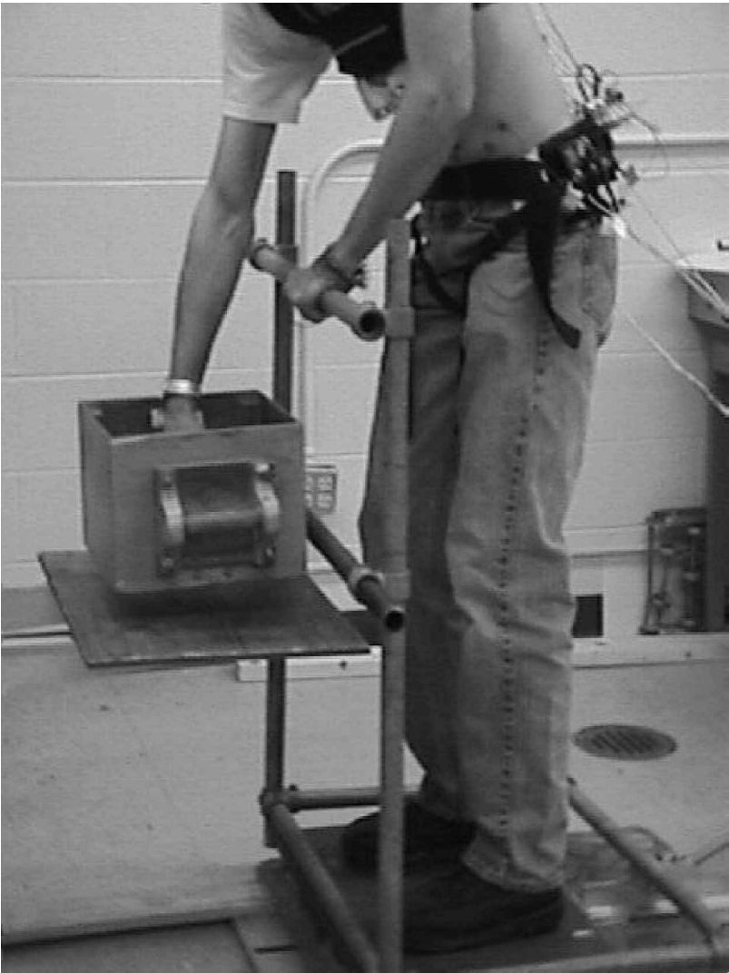
Figure 3. One-handed supported condition when standing on two feet from lifting the upper front region of bin.
