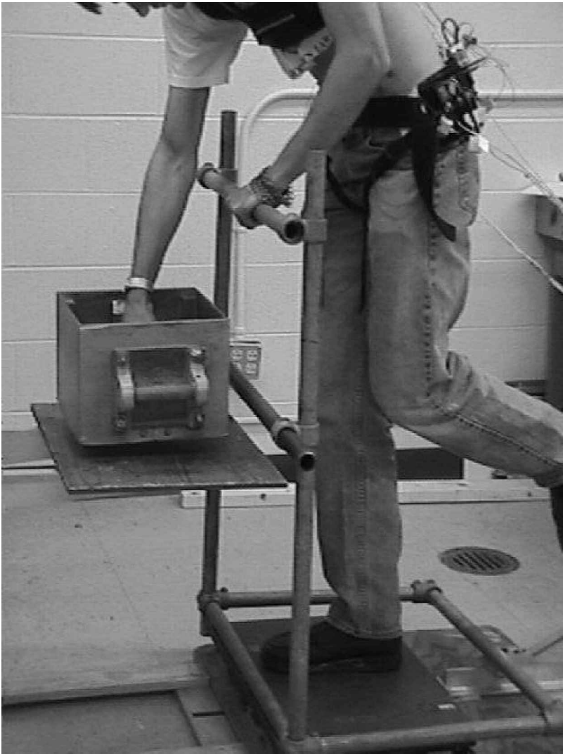
Figure 2. One-handed supported condition when standing on one foot from lifting the upper front region of bin.
