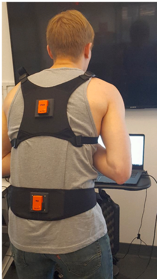
Fig. 1. Clinical Lumbar Motion Monitor uses wearable motion sensors mounted on chest and waist harnesses to quantify functional performance of patients in clinical settings.
