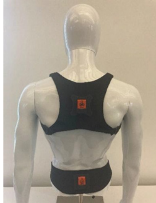
Figure 1: IMU sensor configuration for Lumbar Spine Motion Assessment
